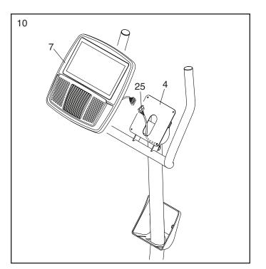
11. **Tip: Avoid pinching the Main Wire (25).** Attach the Console (7) to the Handlebar (4) with four M4 x 16mm Screws (2); **start all the Screws, and then tighten them.**
